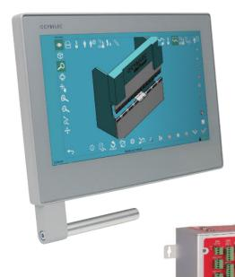
VisiTouch Pac MX is a 3D graphical numerical control for CNC press brakes with a new solution all-in-one:
